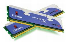
Microsoft Word your computer reads the files for the program off the hard drive and transfers them into RAM. As you use the program the files needed are read quickly from the RAM.
